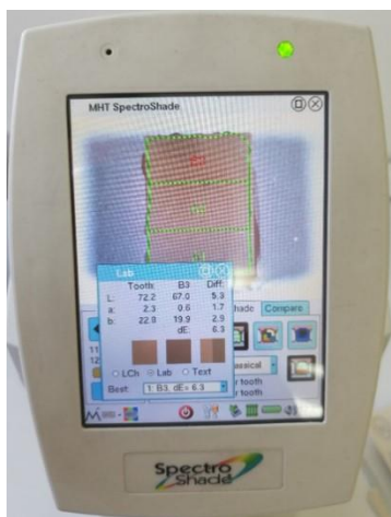
Figure 4. CIELab coordinate measurements by a dental spectrophotometer.
